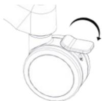
Press down on brake to lock casters, and push brake up to release.
