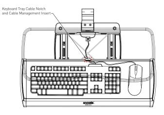
Replace the the keyboard tray (if needed) and place the mouse and keyboard into place.
