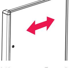
Depth Adjustment: Turn rear spiral-tech cam screw to adjust door position.
