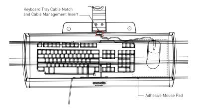
Run the mouse and keyboard cables through the keyboard notch letting them hang out of the bottom of the keyboard tray.
