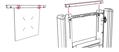
Loosen and remove thumb screws below bottom bracket then remove bottom bracket from unit. (Keep parts for future use)
