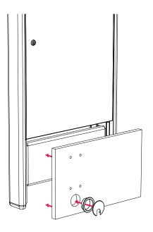
**STEP 1** Place the cable management cap into place
