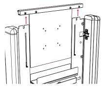
Attach CPU to vesa plate (Screws provided with CPU).
